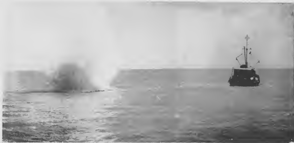
FIVE FEET below the surface of the water an explosive charge is detonated from the near-by "shooting ship." Shock waves, bouncing off the underlying floor of the Gulf of Mexico, are transmitted to the "instrument ship" and recorded on a seismograph. Geophysicists can "see" far into the Gulf bed by interpreting the seismograph recordings. The maximum "shot" permitted is 40 pounds of dynamite.
